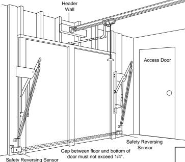
**Closed Position** Rail Bracket Rail Assembly Header Trollev Door Bracket Emergency Release Rope & Handle Straight Curved Garage Door Door Door Arm Arm Header Wall
