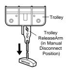
Lockout position (Manual disconnect)
