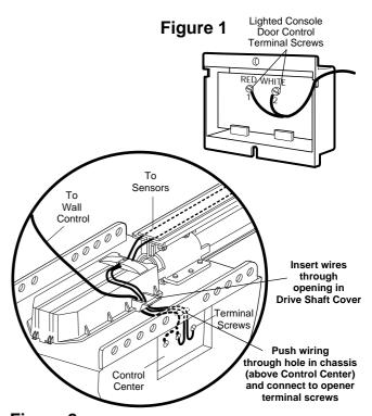
Figure 2 WIRING TO CONTROL CENTER
